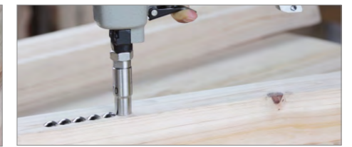
Step3 Actuate the trigger to shoot
